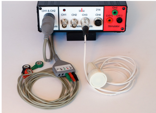
Figure HH-2-L3: The ECG cable and event marker connected to an IWX/214.
